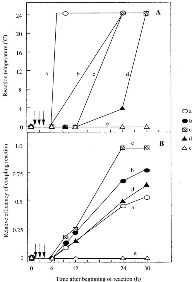
Fig. 2. Temperature schedule for the coupling reaction of CSI and EAH Sepharose 4B with EDC (A) and the relative efficiency of the coupling reaction (B). The schedule c resulted in the highest efficiency. Arrows indicate the addition of EDC three times.
